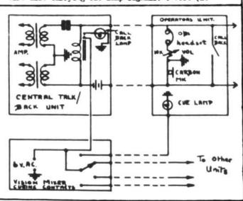
least) one lamps should be used with one side grounded. The microphone and headset should be in series and wired to a terminal block (see below). For call-back a shorting key may be placed across the speech lines.
