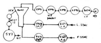
tube (lkV) is generated by a Cockroft-Walton multiplier from the low-level HT transformer. The second video stage acts as a high peaker, and the 2.5 Mc/s bars are easily seen on the final picture. The choice of scanning tubes was governed by what was in the junk box at the time!
